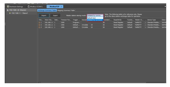
The program trigger mode for the channel is enabled by default. User can use "program-controlled triggering" to activate the channel via 'ModbusTCP\_LinkRun' and deactivate it via "ModbusTCP\_LinkStop".
