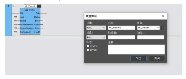
Set the MC\_Power function block input pin
