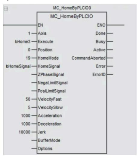
MC\_HomeByPLCIO function block test (following are the sequential steps)
