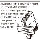
①向上拉动双向联动卡扣 Pull up to unlock the DIN rail mounting latch ②取下耦合器 Detach the coupler
